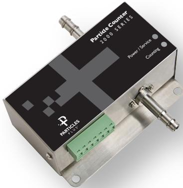
The Particles Plus 2501-4 Remote Particle Counter measures 0.5  $\mu\text{m}$ , 0.7  $\mu\text{m}$ , 1.0  $\mu\text{m}$  & 5.0  $\mu\text{m}$  with a flow rate of 0.1 CFM (2.83 LPM). Integration is easy into a real-time monitoring or building management system via Modbus RTU or ASCII. The 2501 models are the smallest remote particle counters in the market and have easy mounting options. The Particles Plus 2501-4 units comply with ISO 21501-4 and include a 2 year limited warranty.
