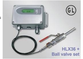
a = 0 corresponds to water-free oil, while a = 1 describes fully saturated oil. a measurement with HLX36 transmitter series is based on the outstanding long term stability and resistance to pollution of the capacitive sensor elements series HC.
