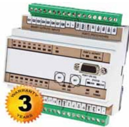
The E-101 is a extension module for family of telemetry modules. It is optimized for use in advanced measurement systems equipped with 12/24V power source. Additionally, it can act as a universal I/O station with galvanically isolated RS232/485/422 Modbus RTU interface. The ability to run local control program allows to use E 101 module as freely programmable PLC.
